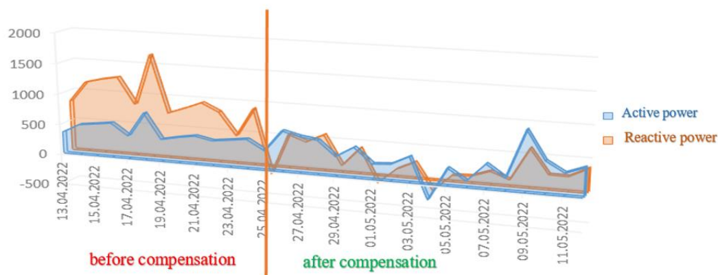
Figure 4 Power consumption of a light industrial enterprise before and after compensation.
