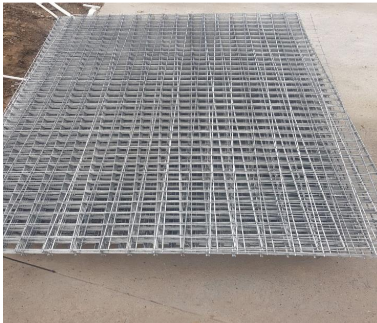
Figure 1. A part of a metal fence when making gabions
