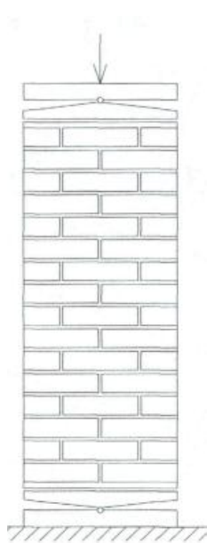
Fig. 2. Testing scheme for brick columns.
