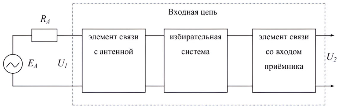
Fig.3. Generalized block diagram of the receiver input circuit.
