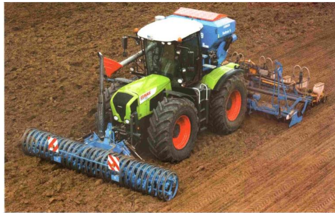
Figure 1. Soil loosening and seeding unit combined with Claas Xerion model tractor.
