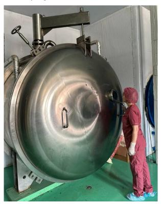
Drying dried plums in a frozen state under vacuum, the moisture in them turns into vapor in the form of ice, bypassing the liquid state, this process is called sublimation. Freeze-drying of products is mainly carried out at low temperature and high vacuum. The study and testing of freeze-drying regimes is carried out in an experimental device with a productivity of 3-5 kg of raw materials per cycle.
