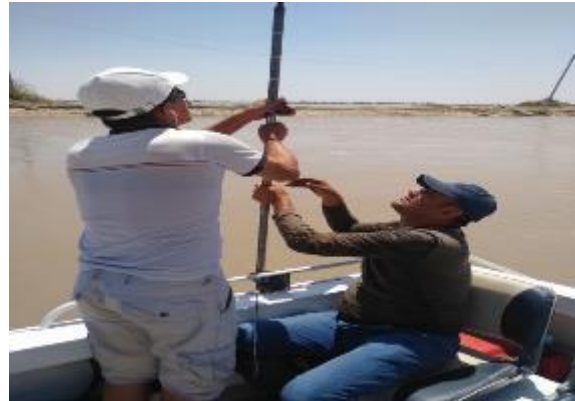
Figure 4. Preparation of hydrometric bar and depth measurement works
