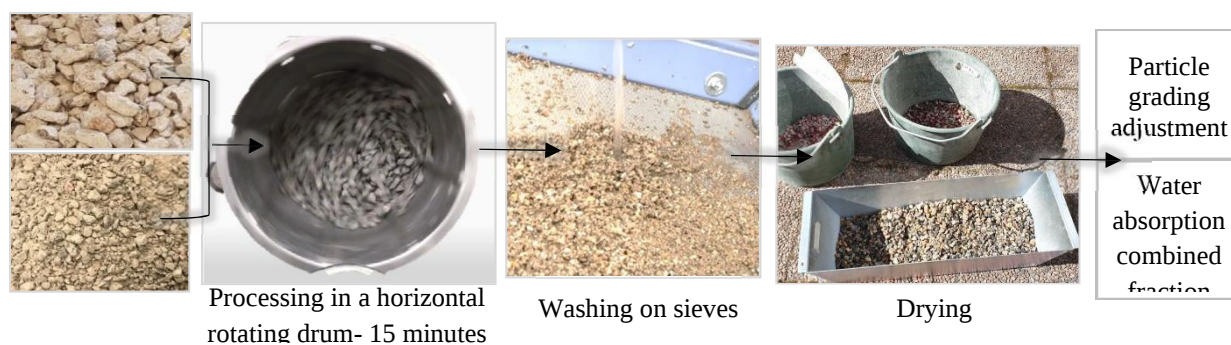
Figure 2. Mechanical pre-processing of CCA for 50% and 100% CCA replacements
