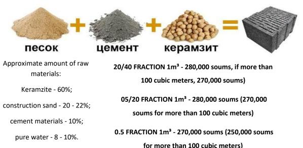
The following are the materials used in the production of lightweight concrete based on artificial filler expanded clay, which has led to a decrease in the cost of concrete when using expanded clay produced in Bandikhon district of Surkhondarya region.
