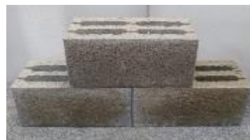
Figure 1.4. Wood-cement block standard dimensions; 190x190x390mm[4]
