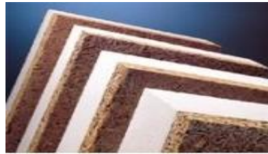
Fig.1. 2. Wood-cement slab with insulation layer; standard dimensions; The size of polystyrene foam is 2000x500x135mm; 2000x500x100mm [4]
