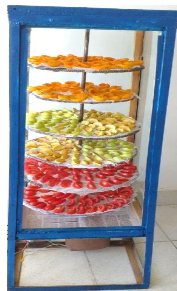
Figure 1: General view of the solar dryer.1 transparent glass; 2nd air-conditioning pipe; 3rd product base (paddon) space, engine that rotats paddies with 4 products installed; 5th ventilator.
