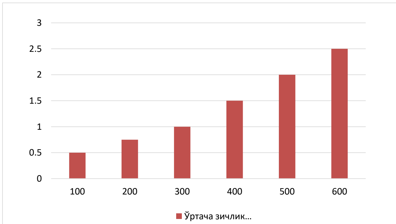
Indicators of changes in compressive strength of polystyrene concrete of different densities.
